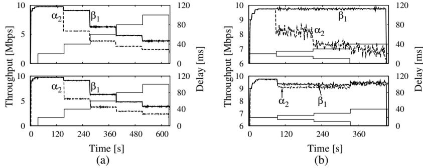
**Fig. 3.** Throughput evolution for different delay settings on the forward (top) and backward (bottom) path: (a) average delay increases over time, delay is equal for all packets (b) average delay is constant over time, delay variance increases over time.
